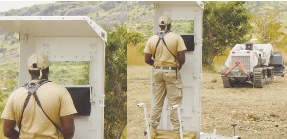
A protective shield protecting the operator of a remote-controlled demining machine
