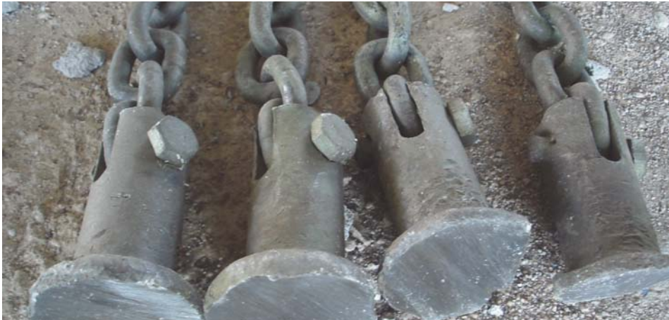
A chisel hammer (tungsten coated)
