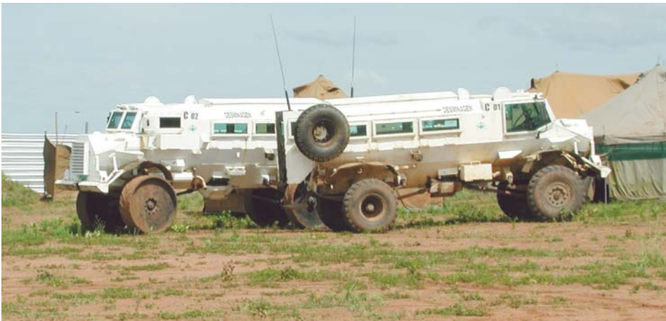
The Casspir MPV: one fitted with steel wheels and one with rubber tyres
