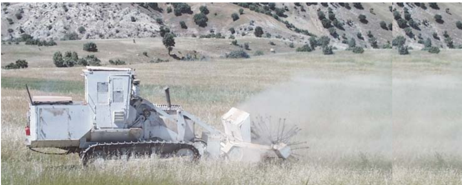
A locally constructed flail in the Kurdistan Region
