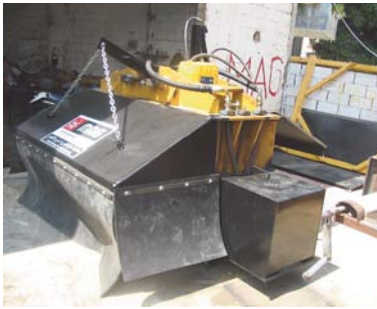
The flail adapted by MAG in Lebanon with rubber mats to reduce dust and throw-outs
