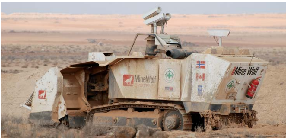
The Mini MineWolf fitted with cameras to operate in dusty conditions
