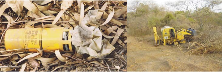
A BLU-97 cluster bomb | A demining machine destroyed by an AV mine
