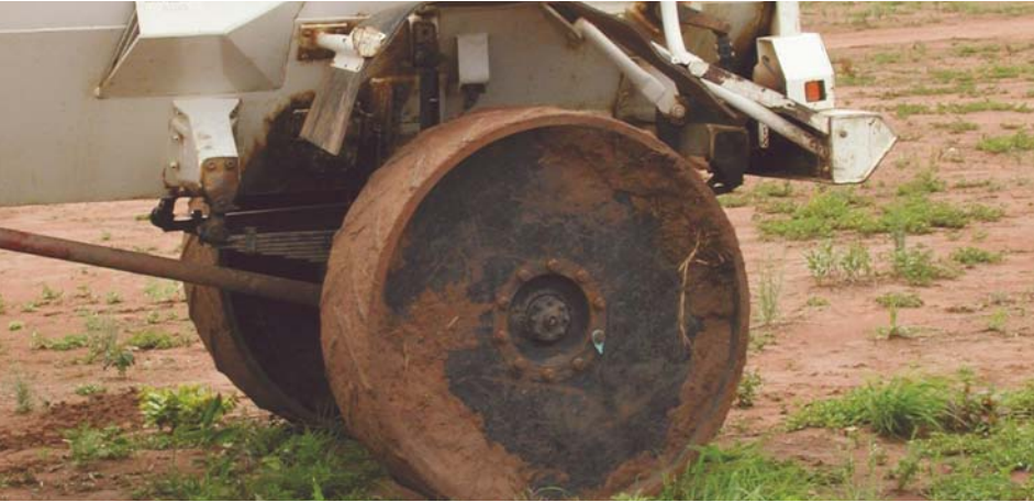
A Casspir fitted with steel wheels
