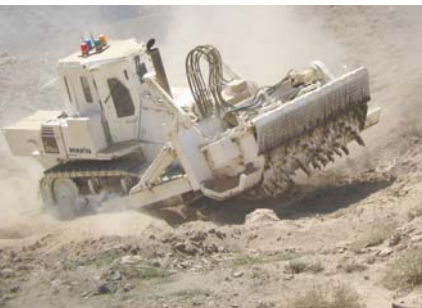
The Komatsu Bulldozer D85MS-15 tiller system in Afghanistan
