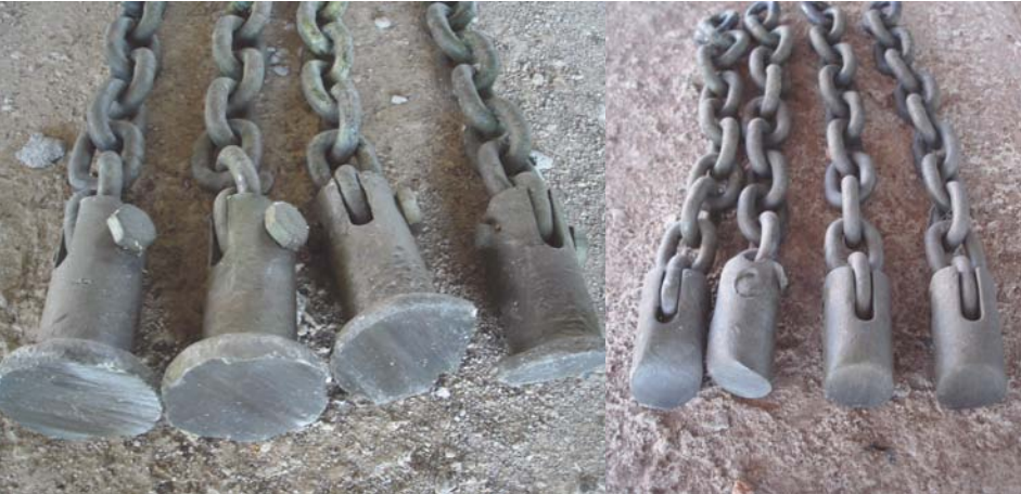
A tungsten-coated hammer after two hours of flailing
