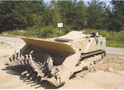
A light tiller which can also act as a flail – the MV-4
