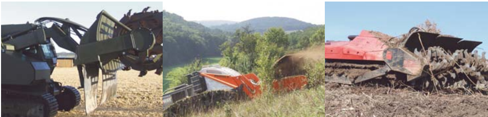
Three machines capable of using a combination of tools | The Armtrac 400, the Bozena 5 and the MV-10
