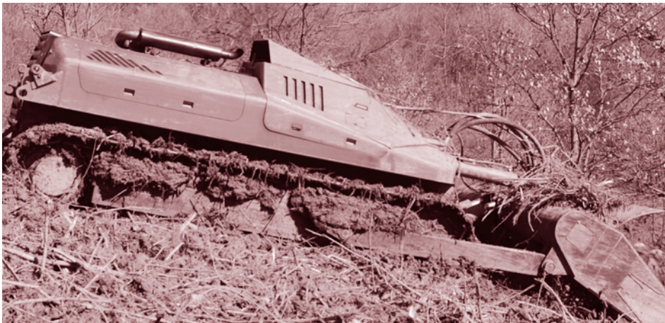
Typically prime contractors will subcontract for mechanical demining
