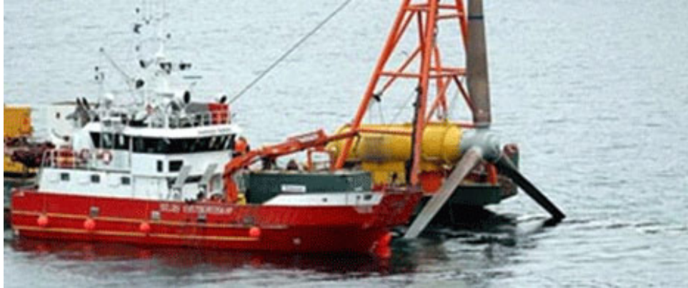
Figure 3.21 Prototype tidal stream unit Hammerfest Strøm (parent company Statoil) Source: Internet Source 75.
