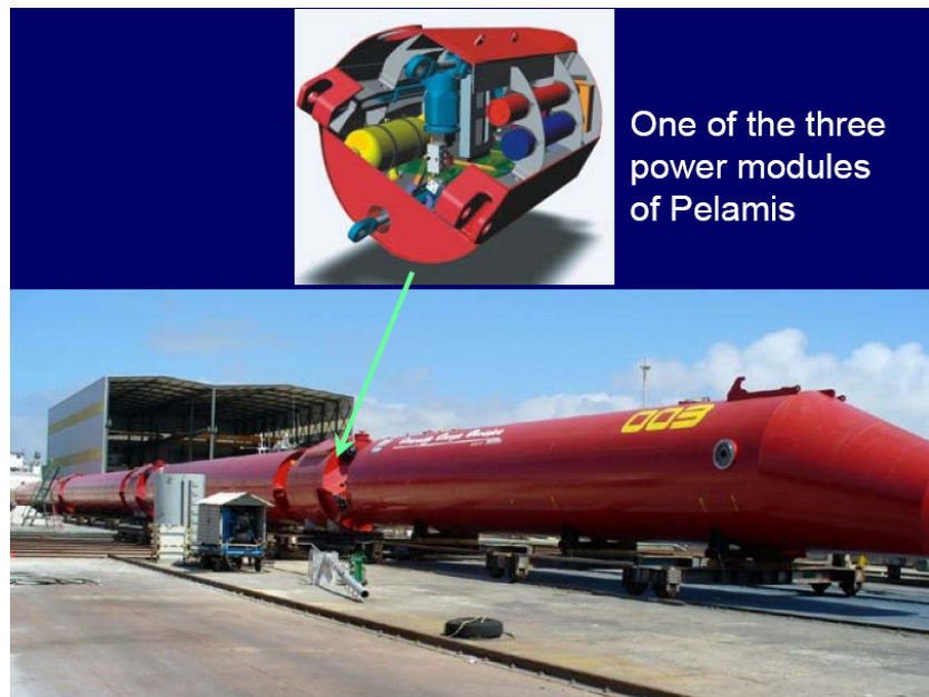
Figure 3.15 One of three sections of a Pelamis module (Aguçadura, Portugal)
