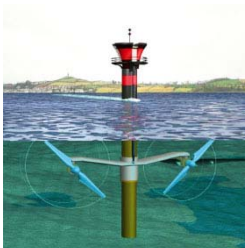
Figure 3.20 SeaGen tidal power (artist impression), Marine Current Turbines Ltd Source: Internet Source 73.
