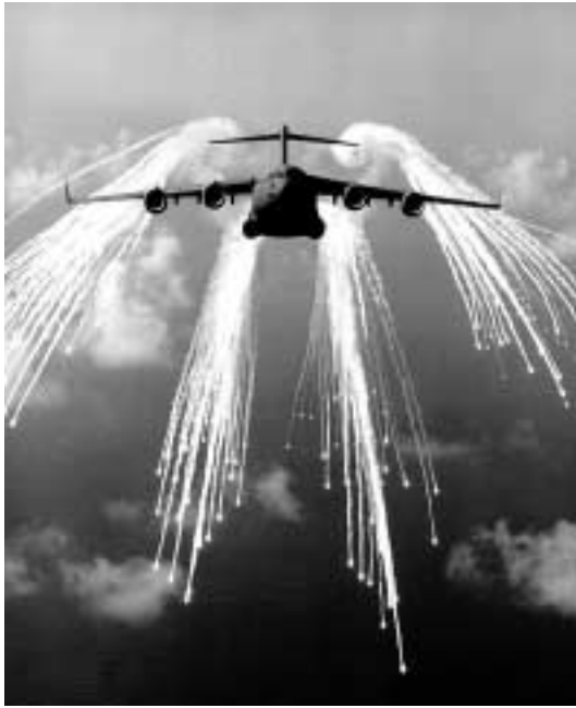
The C-17, here deploying infrared missile countermeasures, can enter environments too dangerous and austere for airliners.
