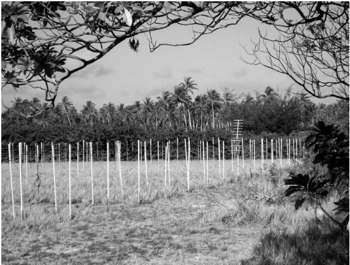
Ionospheric forecasts improve war-fighter communication efficiency. The Scintillation Network Decision Aid antenna, located on Kiritimati Island (Christmas Island), Republic of Kiribati, monitors geostationary satellite communication signals to determine the effects of ionospheric turbulence. (US Air Force photo)
