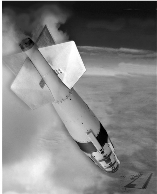
Figure 1. The Joint Direct Attack Munition (JDAM). Widely used during Iraqi Freedom, the JDAM uses the global positioning system (GPS), combined with an inertial system for navigation. Once released, the bomb guides to its target regardless of weather. (From the Boeing Company.)
