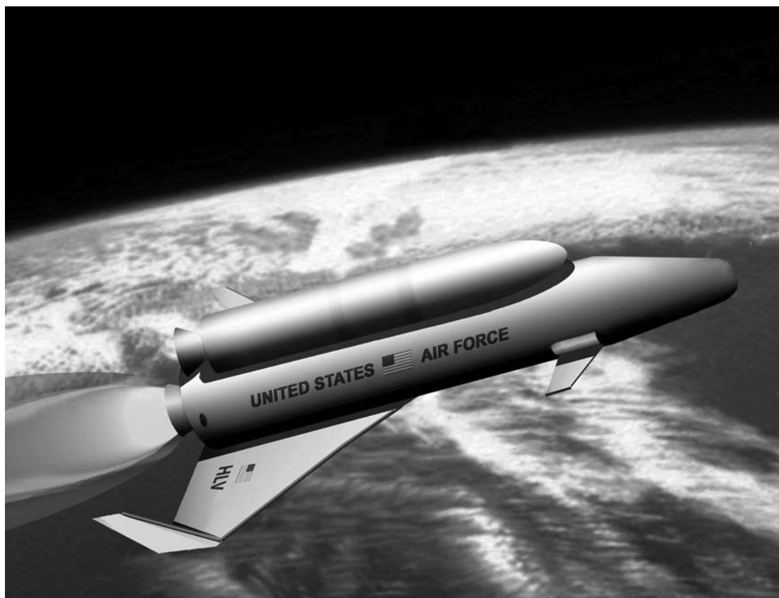
Figure 5. ARES vehicle. The ARES concept calls for a vehicle with a reusable first stage and expendable upper stages (also known as a hybrid launch vehicle). (Courtesy USAF.)
