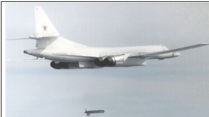
A Tu-160 “Blackjack” supersonic heavy bomber launching a Kh-55SM 385 (AS-15B “Kent”) cruise missile from its aft bay. Source: Carlo Kopp, “Soviet/Russian Cruise Missiles”, Air Power Australia , August 2009, http://www.ausairpower.net/APA-Rus-Cruise-Missiles.html .
