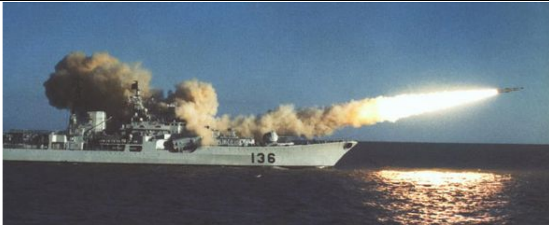
The Project 956E Hangzhou (No. 136) destroyer of the PLA Navy firing a 3M-80E Moskit (SS-N-22 "Sunburn") supersonic surface-to-surface missile. Source: http://www.china-defense.com/smf/index.php?topic=176.0 .
