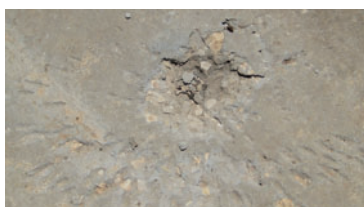
Strikemark DPICM (Dual-Purpose Improved Conventional Munitions) M-77
