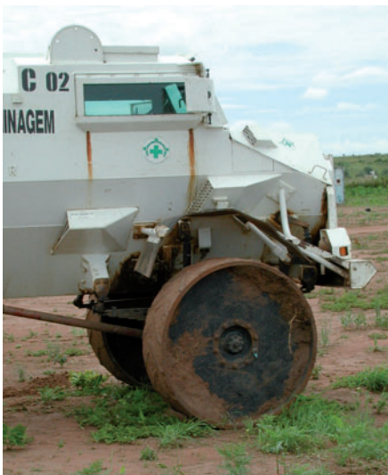
Casspir mine-protected vehicle with steel wheels
