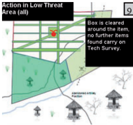
FIGURE 10 | Procedure when an item is found in the low threat area
