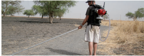
Sample being taken for the MECHM Explosives and Drug Detection System (MEDDS)
