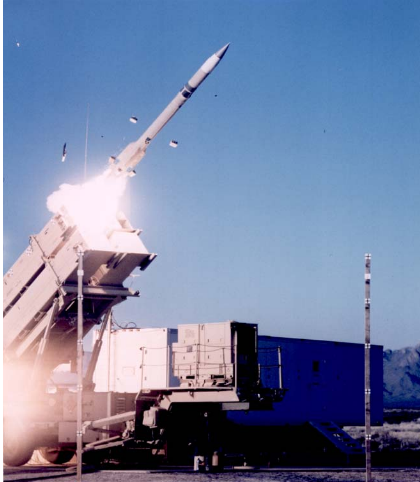
Figure 1. The Ballistic Missile Defense Organization and the U.S. Army conducted a successful test of the Patriot Advanced Capability-3 (PAC03) missile at White Sands Missile Range, N.M., February 5, 2000. The PAC-3 missile is a high velocity, hit-to-kill missile and is the next generation PATRIOT missile being developed to provide increased defense capability against advanced tactical ballistic missiles, cruise missiles, and hostile aircraft. The PAC-3 missile uses kinetic energy (i.e. “hit-to-kill” to destroy targets rather than employing a high explosive warhead. It is the basis of the U.S./German/Italian, and now NATO, theater missile defense system (known as MEADS).
