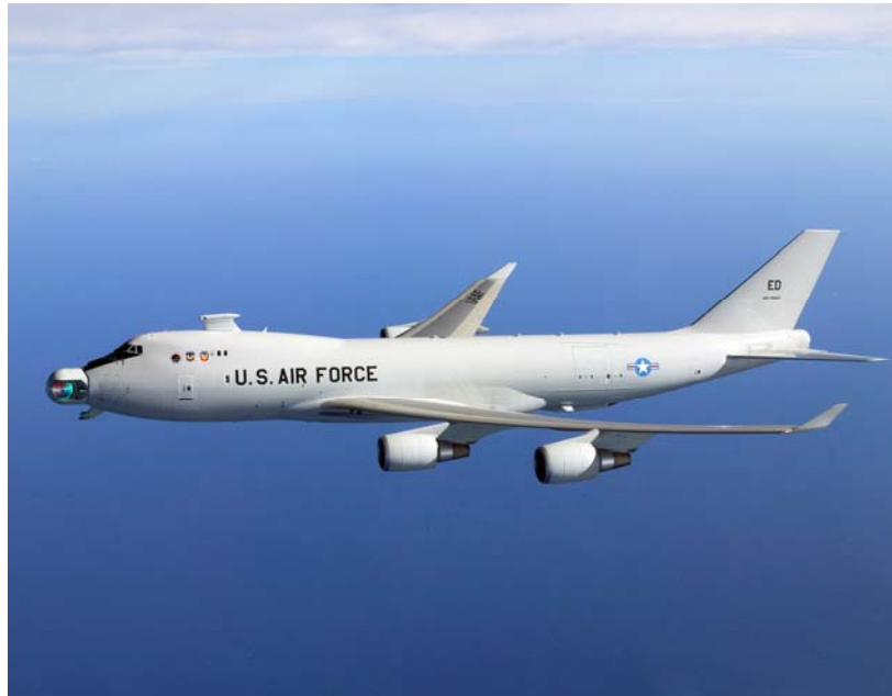
Figure 10. YAL-1 Airborne Laser (ABL) is a heavily modified Boeing 747-400F fitted with a megawatt-class chemical oxygen iodine laser (COIL). Prior to termination of the program, the Air Force envisioned a fleet of seven aircraft.
