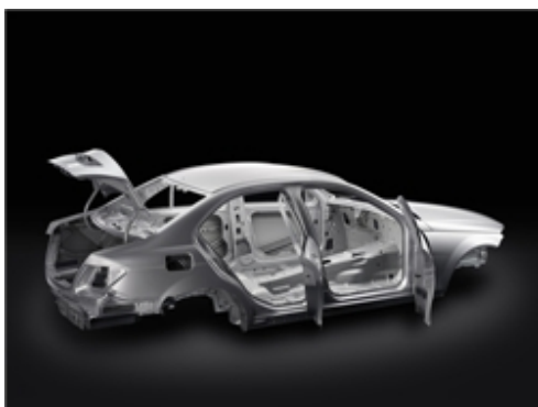
Figure 2 The body-in-white for the 2008 Mercedes C-Class contains 70 percent high-strength steels and 20 percent advanced high-strength steels.
