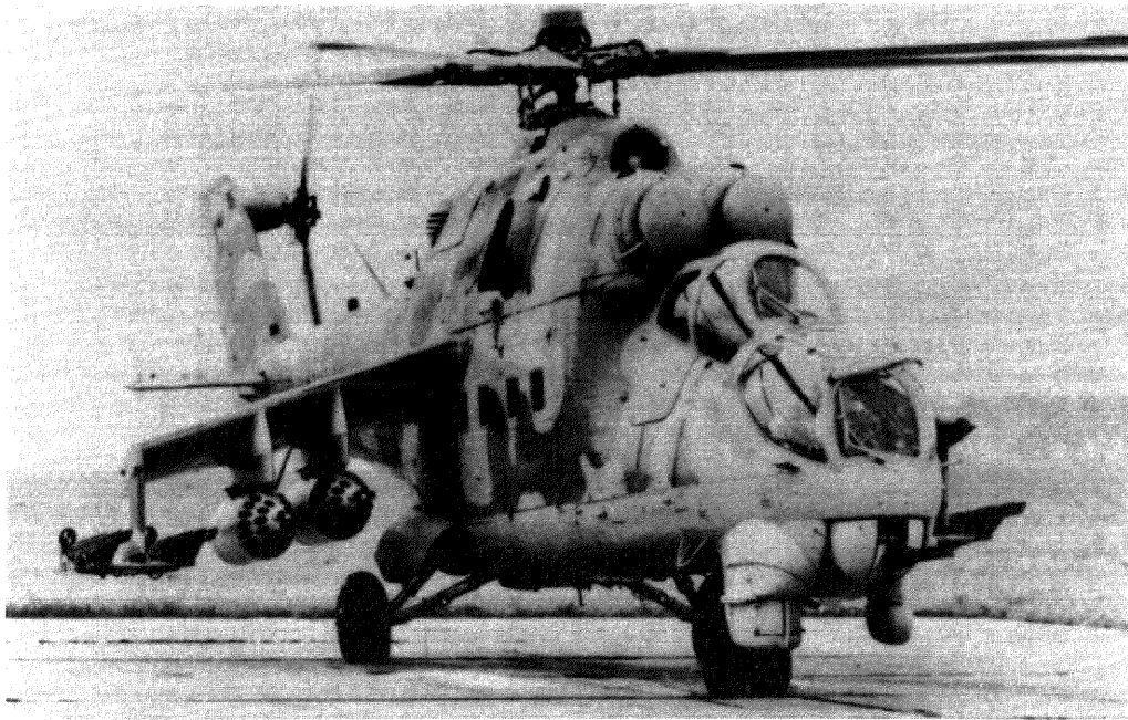
The Mi-24 Hind, the most effective firepower instrument in Afghanistan. Designed as a flying tank, the Hind can carry six passengers and can deliver free-flight rockets, wire-guided missiles, free-fall bombs, and automatic cannon fire.
