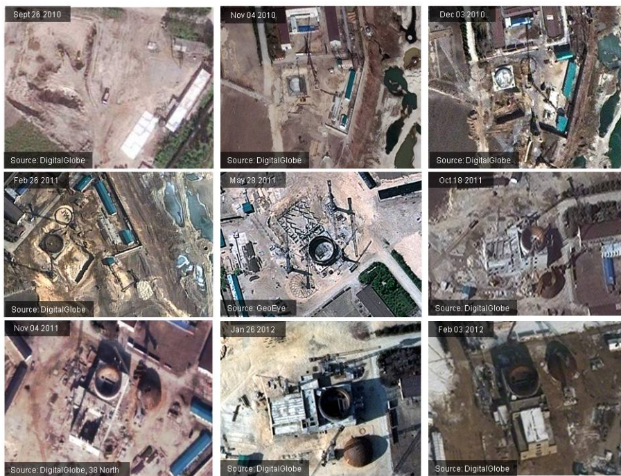
Figure 1 – A time sequence of overhead images of the light water reactor site tracking its development from September 2010 to February 2012. Image Credit: DigitalGlobe and GeoEye
