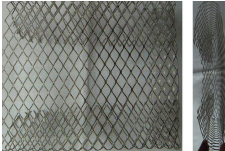
FIGURE 21 | Suggested inlet grid solution covers the whole circular disc of the mouthpiece facing the soil. After Uddqvist and Robertsson.
