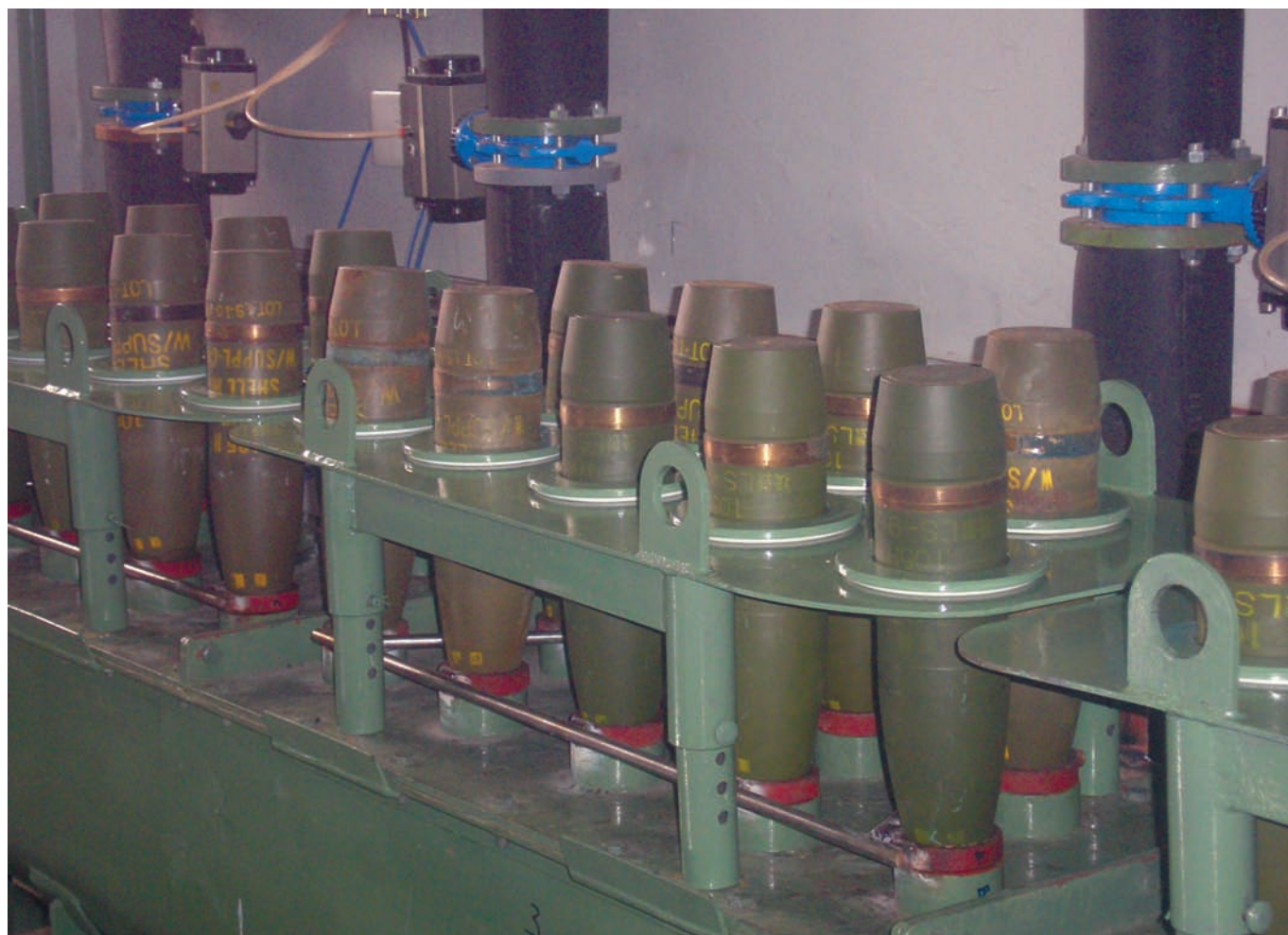
Discharge of TNT-filled projectiles. © Expal Bulgaria
