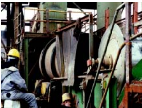
Photo 9: Operation Qeto: Centrifugal and electromagnetic machine that separates ferrous and non-ferrous or non-metallic scrap. Photo credit: South African Department of Defence.
