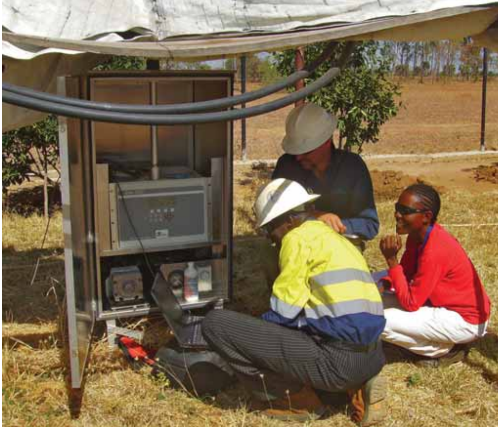
Figure 5: Dust monitoring equipment
