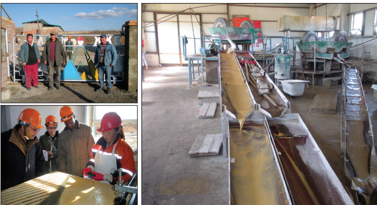
Figure 17: Gravimetric, mercury-free processing plant of the "Hamo Company" in Bornuur, Mongolia. (SAM 2008)
