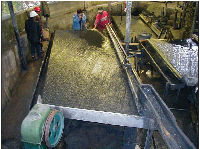
Figure 15: Introduction of shaking tables for gravimetric concentration in the Cotapata Cooperative, Bolivia. (MEDMIN 1998)
