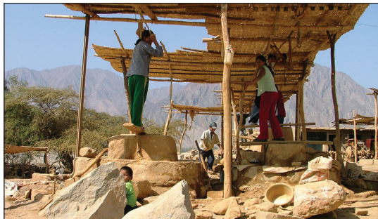
Figure 11: Women miner milling and amalgamating ore in a “quimbalete” processing plant (traditional mortar type mill made out of two big stones) near Tulin, Peru. (GAMA 2003)
