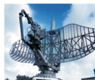
SURVEILLANCE RADAR ELEMENT (SRE)
