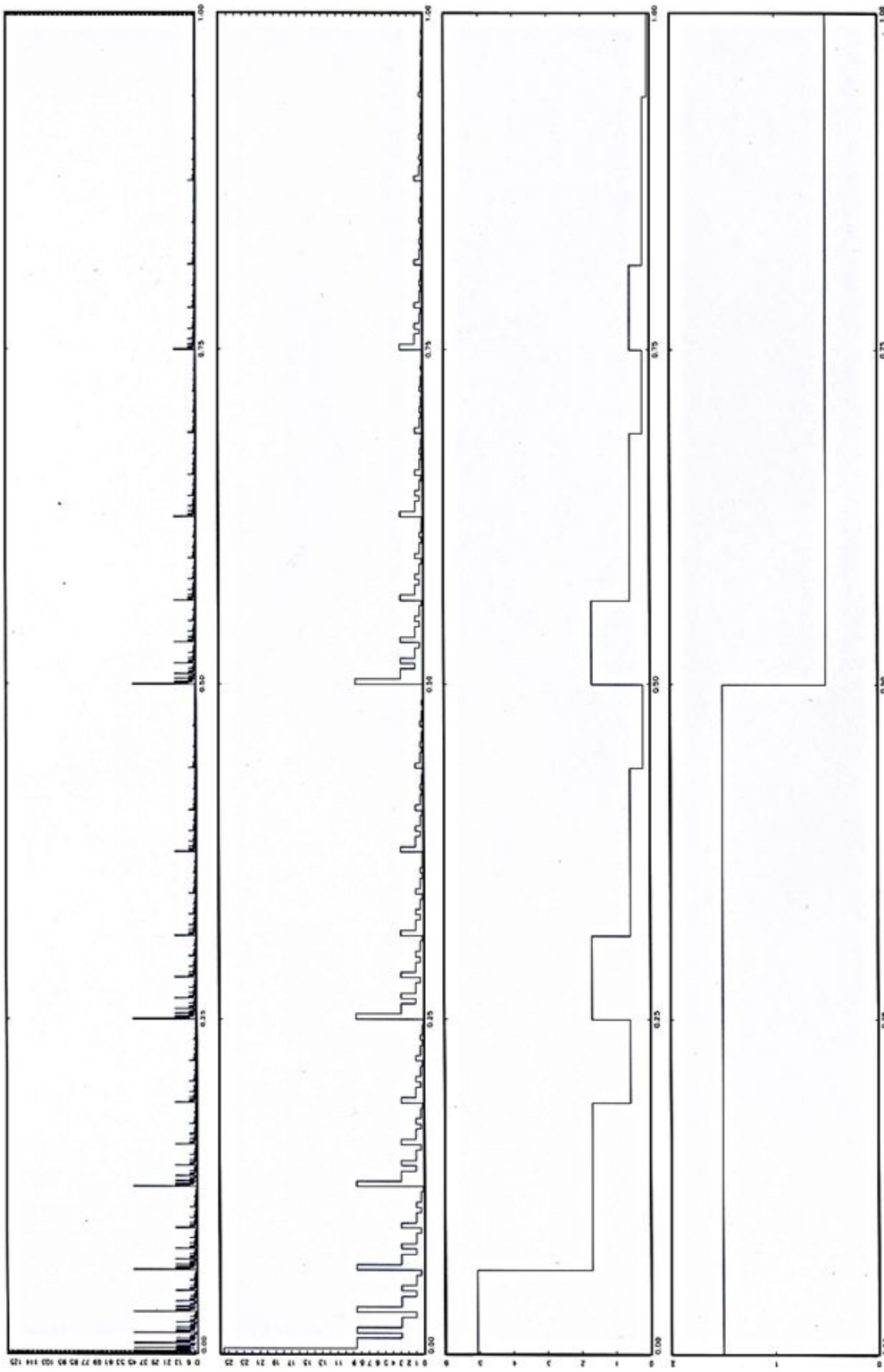
Figure 4: An illustration of the baseline Binomial multifractal cascade. Displayed are the resulting products of multipliers at steps 1, 4, 8 and 12. By moving to higher levels of cascade steps one observes a more and more homogeneous distribution of the mass over the interval [0, 1] .
