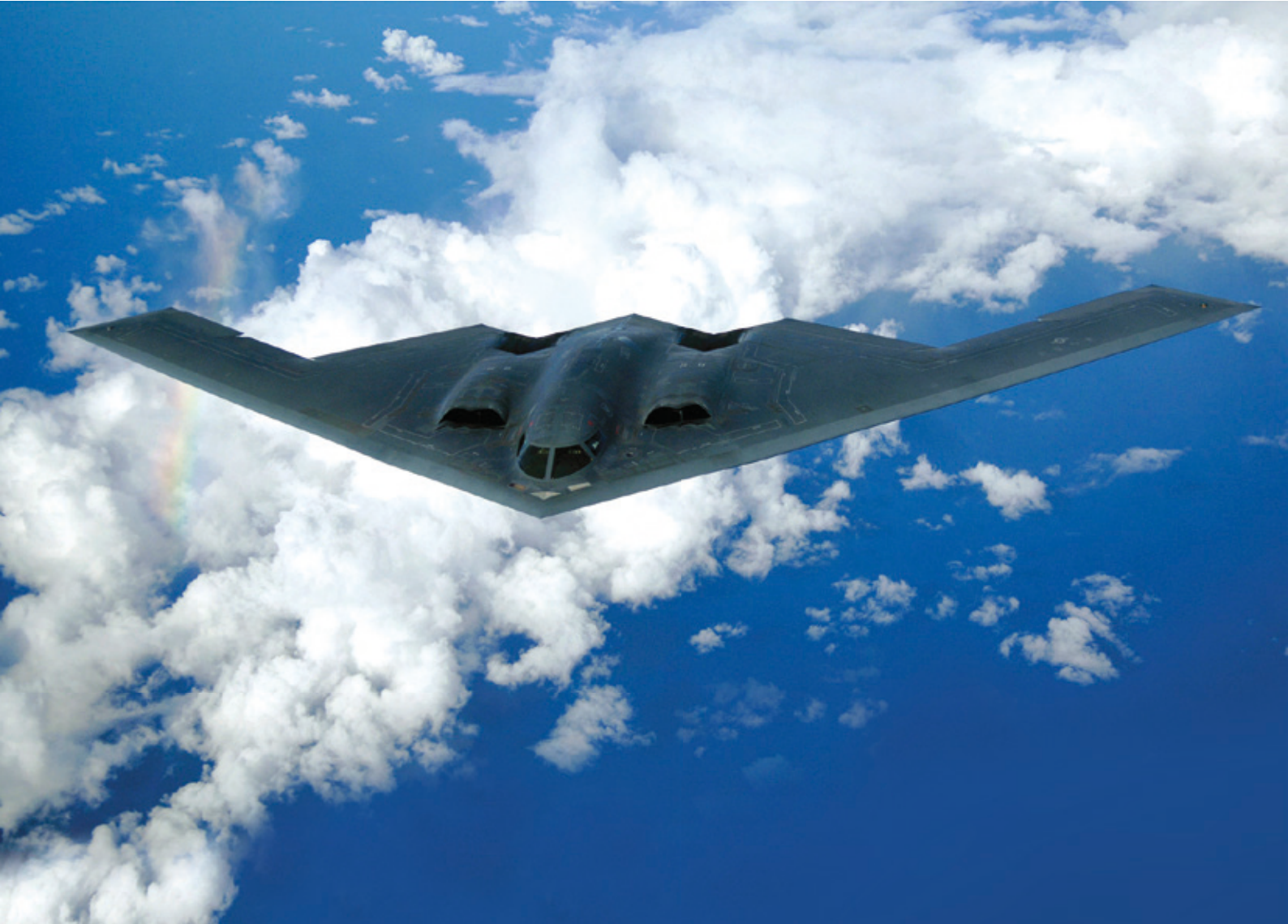
The B-2A Spirit strategic bomber, also known as the Stealth Bomber, can carry up to 16 (1,100kg) B83 nuclear bombs. Copyright: U.S. Air Force photo/Staff Sgt. Bennie J. Davis III.
