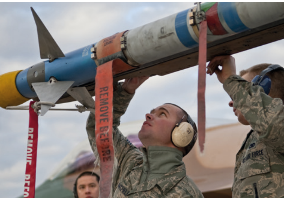
U.S. soldiers secure an AIM-9 Sidewinder air-to-air missile on an F-16 Fighting Falcon aircraft. Copyright: DoD photo by Airman 1st Class George Goslin, U.S Air Force/Released.
