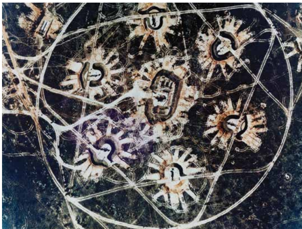
FIGURE 42. TYPICAL SA-2 SITE CONFIGURATION
