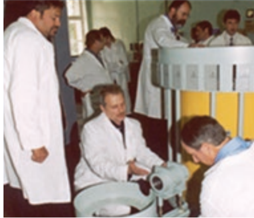
Figure 4. American and Russian experts examine an attribute verification system employing neutron multiplicity counting and high resolution gamma ray spectrometry with information barriers (AVNG) built at Sarov and approved for use in Russian facilities by Russian security authorities (FSB). (Photo courtesy of D. MacArthur, Los Alamos National Laboratory.)
