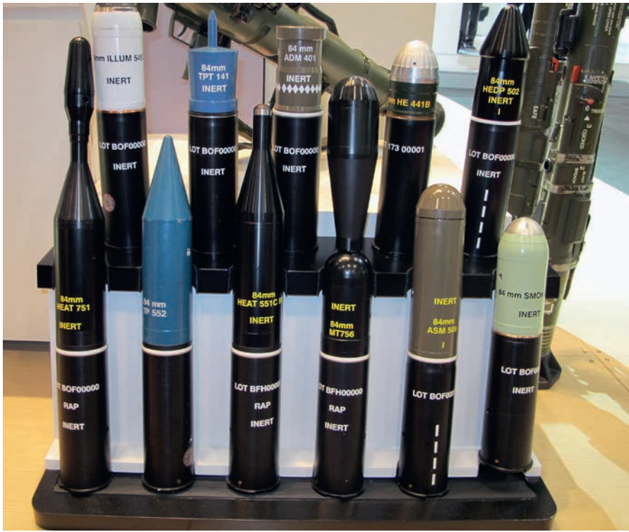
A range of projectiles for the Swedish Saab Carl Gustaf series of recoilless rifles, including HE, HE-FRAG, HEAT, anti-structure, smoke, illumination, and practice rounds. © N. R. Jenzen-Jones/ARES
