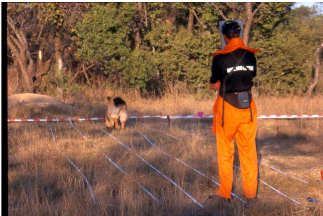
Fig. 5. Guide lines set out for searching. One set of guide lines is shown. The dog is taught to search up and back one lane at a time. Minefield marking tape can be seen at the edge of the search area. Photograph courtesy of I. McLean, GICHD, 2001a.
