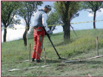
Figure 4. Manual deminer working with metal detector (code e.g. MD)
