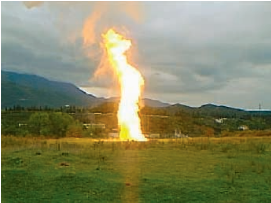
Effect of unconfined propellant ignition: only 50 kg of propellant is burning.
