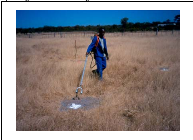
Figure 2. Producing a matched pair of filters in a test minefield. The sampler carries a backpack on which the vacuum pump is mounted, and walks slowly forward passing the tube over the ground in an arc.
