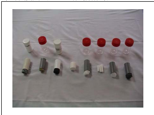
Figure 3b. CSIR filter (top), original Mechem filter (middle) and IVEMA filter (bottom).
