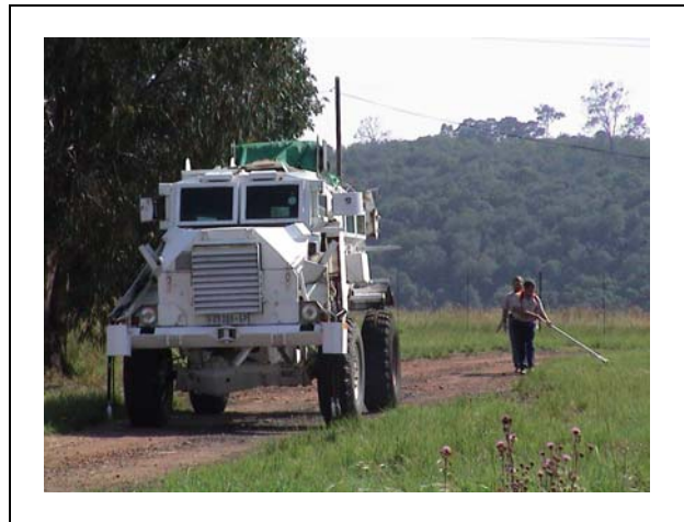
Figure 1. A sampling team working behind a Casspir mine protected vehicle. The vehicle also carries front-mounted vacuum tubes.
