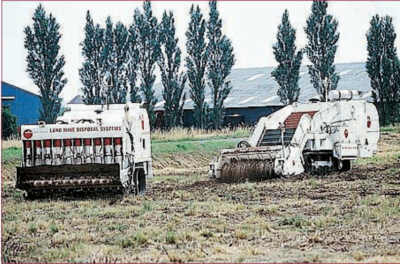
The Redbus Land Mine Disposal System consisting of the Bigfoot (left) and Mineworm (right)
