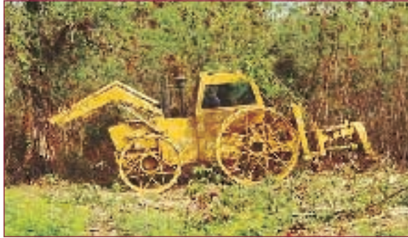
The Pearson Slasher at the rear of the tractor cutting vegetation
