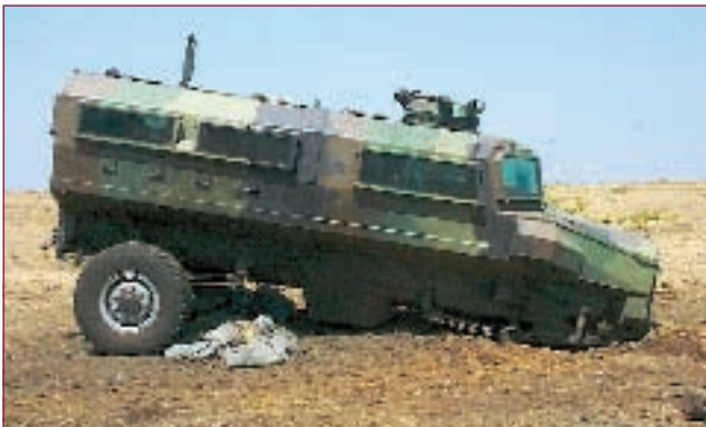
Wer'wolf after detonation of 14kg of TNT under the front axle
