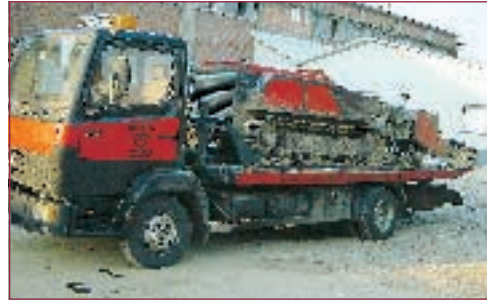
MV-4 mounted on truck
