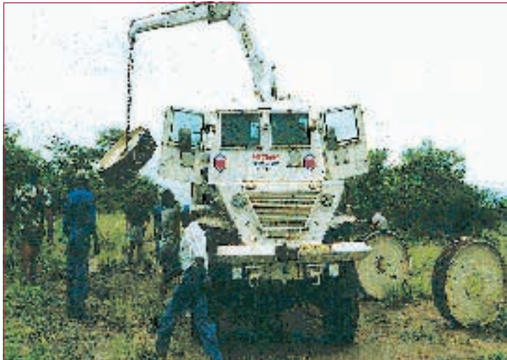
Early version of Casspir mounting steel wheels
