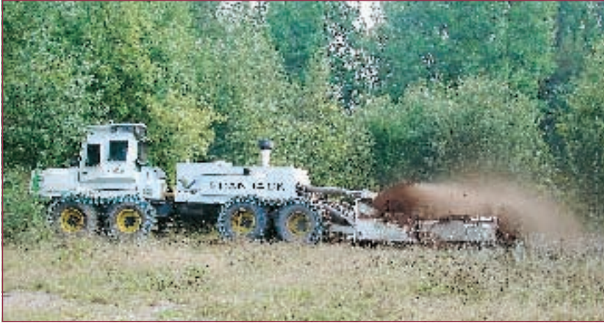
Scanjack operating in overgrown vegetation
