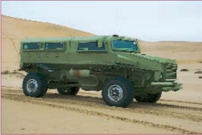
The Wer'wolf MkII Modular Mine Protected Vehicle personnel carrier
