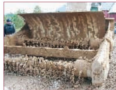
The double flail unit of the Scanjack
