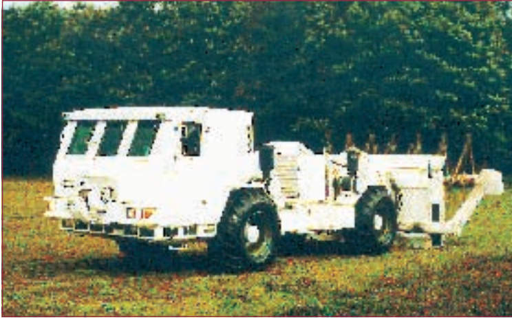
The Hydrema 910 MCV with flail unit
