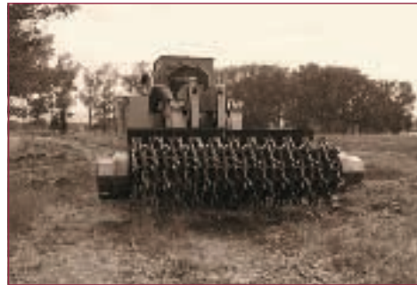
Spitfire tiller unit with carbide metal cutting bits
