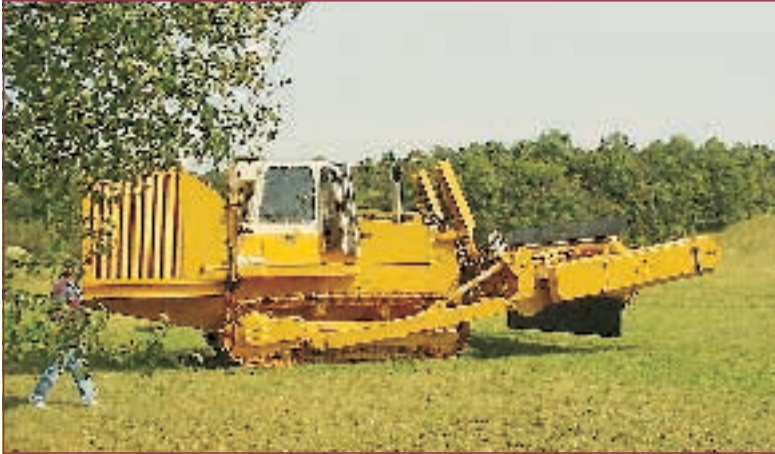
The VIKING system with flail and power pack
