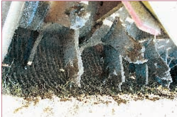
Tilling drum with tungsten teeth
