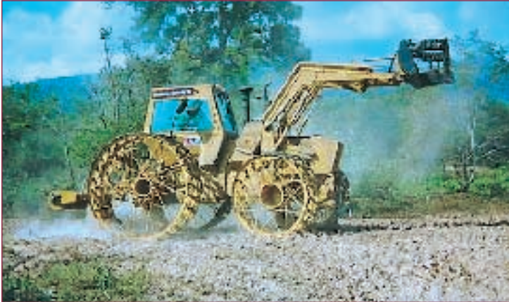
Pearson SDTT with roller and loader
