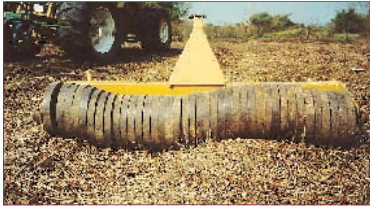
The area reduction roller with its 50 kg discs
