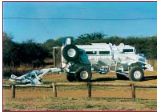
VAMIDS™ mounted on mine-protected vehicle
