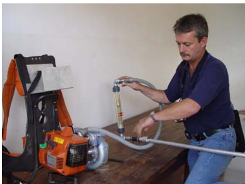
Philip Eskeland (IVEMA) demonstrating a modified sampling machine with integrated gauge at the workshop in Tanzania
