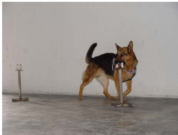
A rest dog licking on the filter to be sure of detection - effectively leaving a clue for the next dog. The result - the next dog may detect the salivary from the first and not the explosive trace in the filter. Clues are difficult to identify and require careful examination of the training and analysis process
