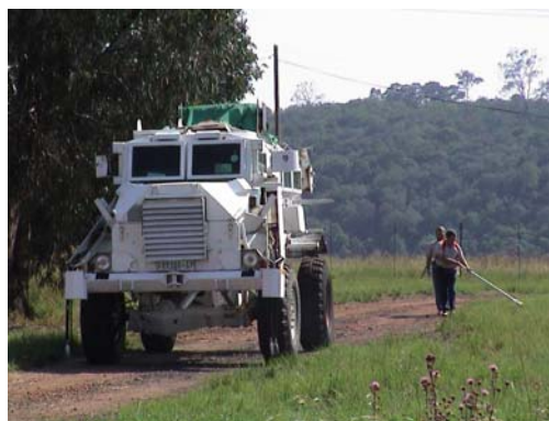
Casspir with an integral sampling system, used in the early days. The filter cartridges are seen hanging to the front of the vehicle. Safe for the operator but offers limited control of the sampling zone. Portable sampling units are used behind, to ensure suction from vegetated areas
