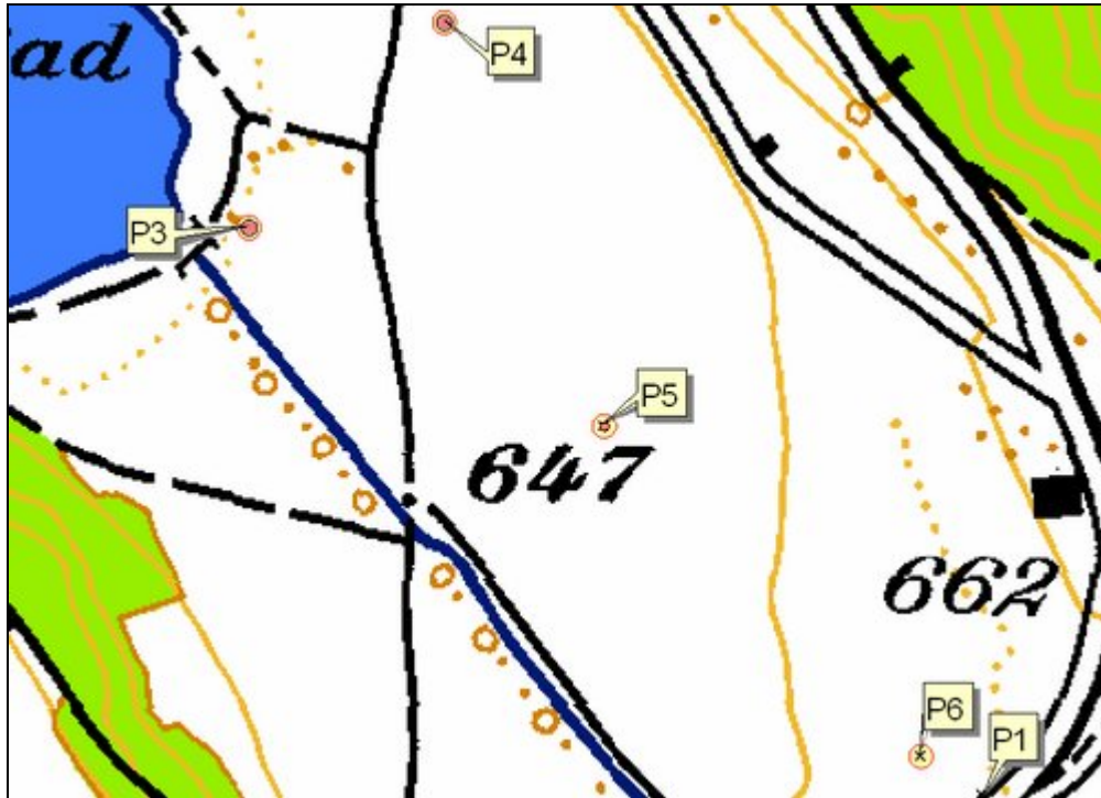
Figure 5. Comparing the accuracy of the two techniques when all distance measurements are made from the reference point (P1). The yellow circles indicate the GPS positioning error and the red circles show the error when measured by the bearing and distance technique.
