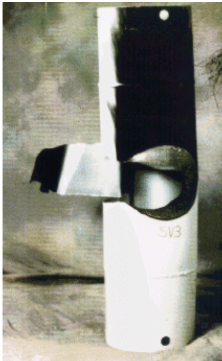
Figure 3. The ABL's missile kill mechanism has been studied in ground tests. Here, a steel vessel similar in dimensions to a SCUD fuel tank is shown after such a test. The laser beam first removed the paint covering the simulated missile. Soot from the paint is visible above the region of exposed metal. Then, the laser heated up the metal skin to the point where the internal pressure caused the tank to rupture. A vertical crack formed first, suggesting failure due to hoop stress. Immediately afterward, the flap, visible on the left, "unzipped." The laser has been dithered in a circular pattern to produce this large region of affected skin. In powered flight, the missile would almost certainly have collapsed after the laser produced such a large hole. Photo source: Phillips Laboratory.
