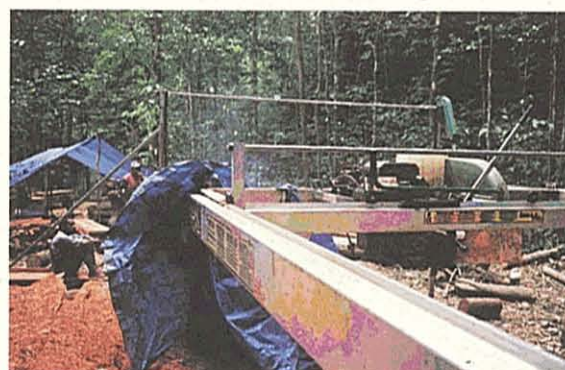
Portable sawmill set up to produce certified timber - PNG
