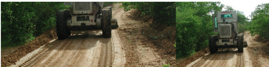
A motor grader used on roads
