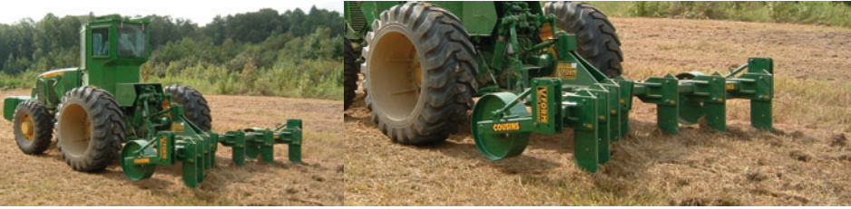
An example of a soil loosener, attached to a Pearson Minefield Tractor
