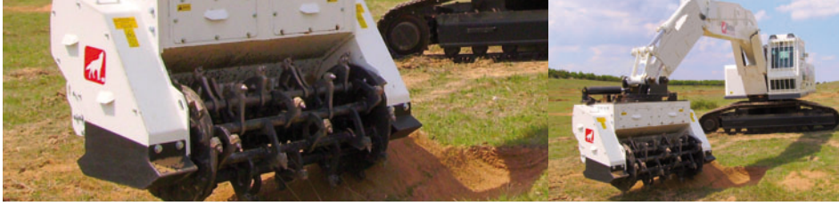
An example of a ground preparation machine | the MineWolf Bagger
